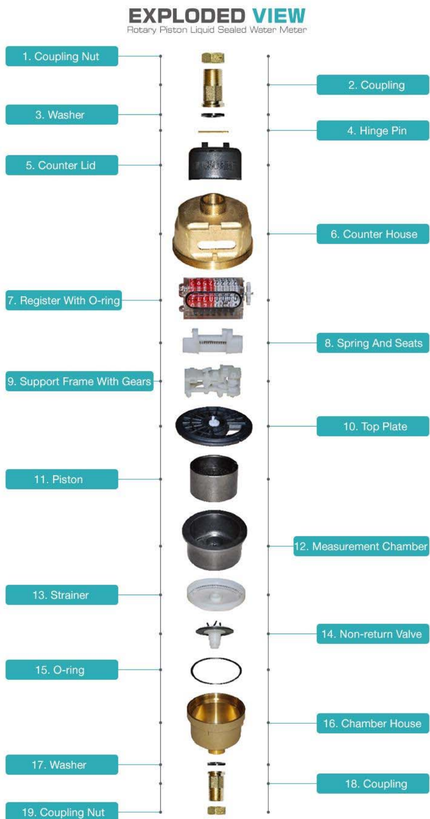
Figure 5.5 Exploded View of Oscillating Piston Meter
