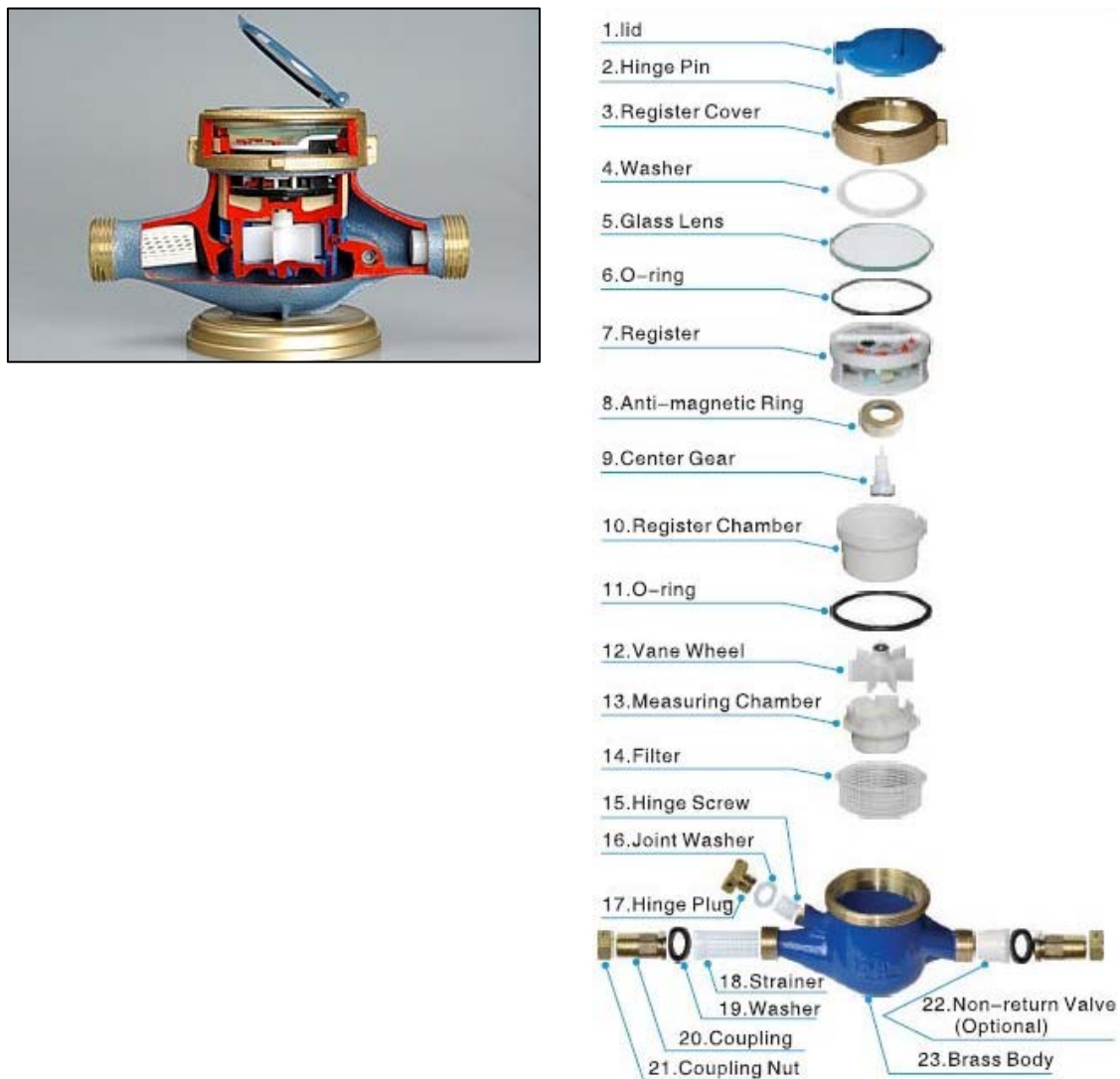
Figure 5.1 Exploded View of Velocimetry Type Water Meter
