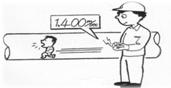
Figure 6.3 Sound velocity in the water-filled pipe
