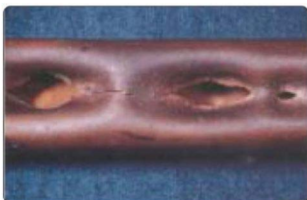
Figure 6.6 Examples of damage caused by water hammer
