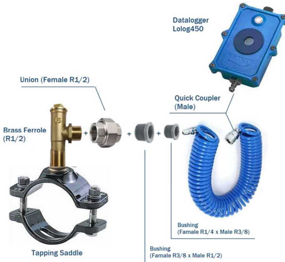
Figure 4.3 How to connect datalogger with tapping saddle
