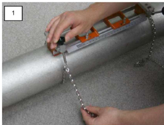
1. Roll chain around the pipe.
