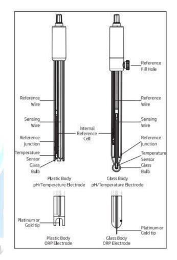
• Place in storage solution for at least 1 hour and re-calibrate before next use.
