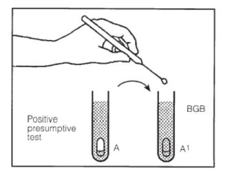
• To confirm the presence of fecal coliforms, incubate the subculture tubes from each presumptive positive tube for 24 hours at 44.6±0.5°C.
