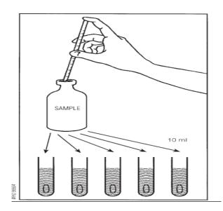
✓ For untreated samples, pipette 1 ml of water into each of five bottles containing 5 ml of broth.
